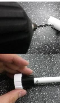
Drill a hole in the end of tube.
