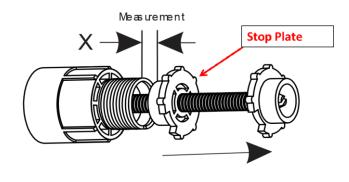
Below shows stop plate half way from stop spring
