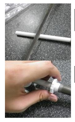
Cut the inner tube same length as spring cutting length.
