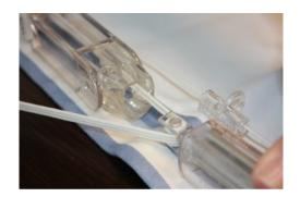
\*Thread exposed cords through top of Handle with curved shape facing lining of shade.
