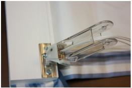
\*Thread exposed cords through Cord Lock Connector - 5 Cords Maximum \*Position 'Cord Lock Connector' over cord lock and into position with small angle edge toward inside, facing left. Insert  $1\ 1/8$ " screw and #40 nut. Push screw completely through connector and cord lock, attach nut until secure.
