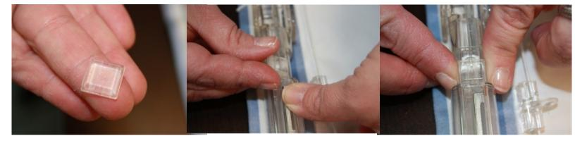
\*Place cord stop at the top of handle where the handle rests when the shade is in the down position. \*Trim excess cord from back of knot to 1/2". We recommend putting a drop of glue on the knot.
